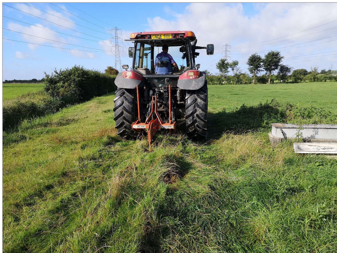
Figure 5.5-4. Mr Andrew Waters, of Cross Farm, mole-ploughing a small part of the Cross Farm; Nash monitoring site to find the lines of the under-drains.
